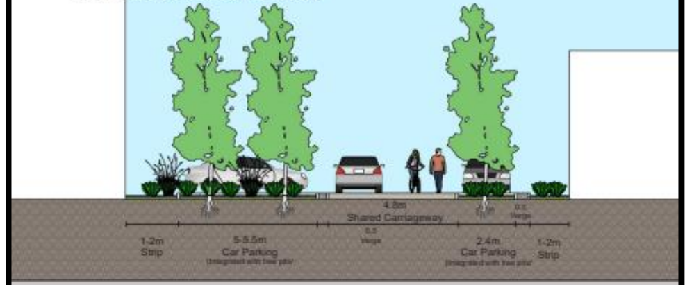
Figure 3.6: Transition zone incorporating landscape/SUDS features which reinforce a gateway to reduce vehicle speeds upon entry to an urban area.
