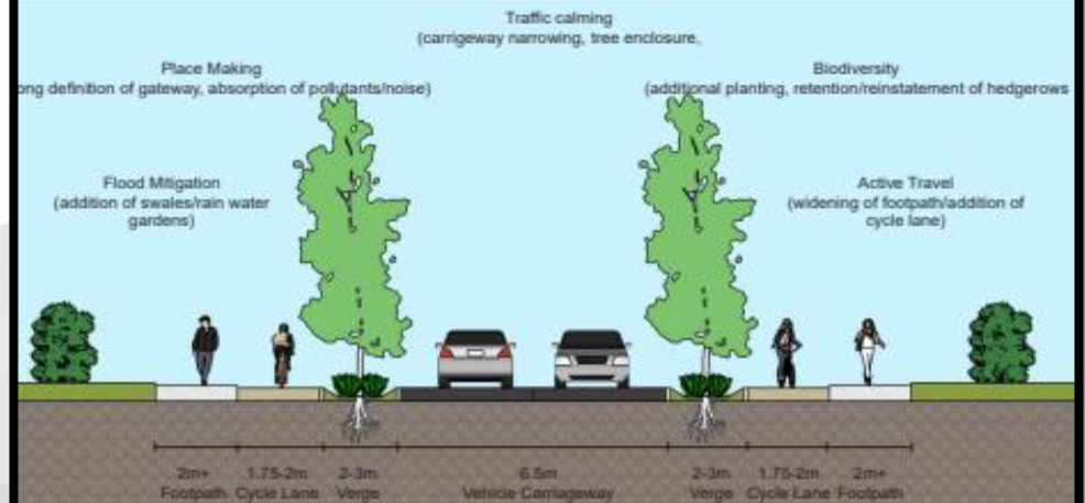
Typical section in Transition Zone - predominantly hard surfaces with limited Active Travel
